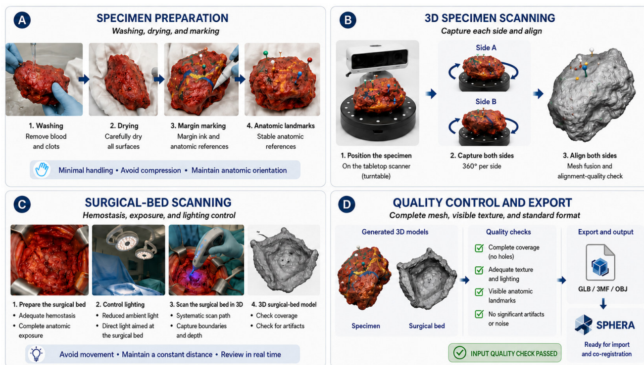
Figure 3. Conceptual representation of the preparation, scanning, and quality-control procedure. Approval labels shown in the illustration refer to operational input checks, not validation of clinical accuracy.
